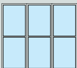
Prepared for site infill (max. 16 kg/m 2 ) resting within the frame Frame in terra brown (RAL 8028)
