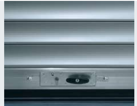
Bottom profile locks from the outside With profile half-cylinder, can be locked from the inside without a key. Operated from the outside via a recessed handle, from the inside via a T-handle. For all shutter widths.
